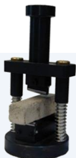
Flexure fixture for square cement specimen tests.
