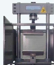
Flexure testing frame with tilting rollers.
