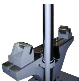
ME 403 + grips 4011ACH + 3 points flexure fixture.
