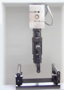
3 points flexure dixture for ME-402 and ME.405
