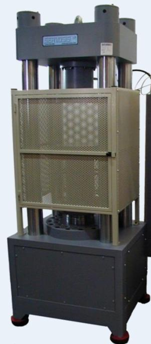
MES machines can be equipped with a simple or a double acting actuator.
