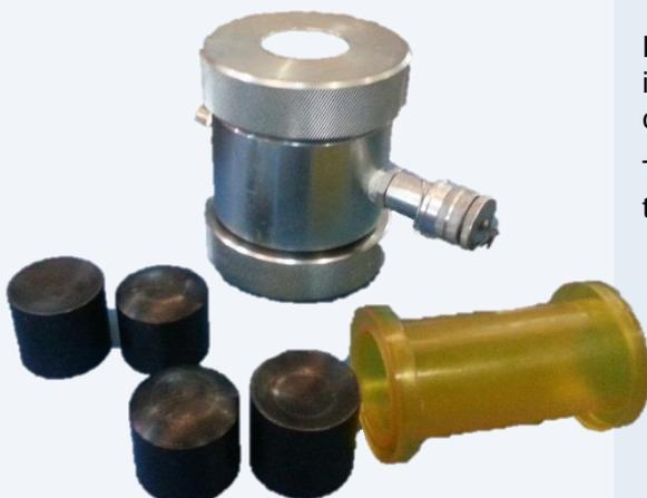
During the test, the lateral pressure application can be constant or increase as the axial force increases, depending on the test method chosen.
