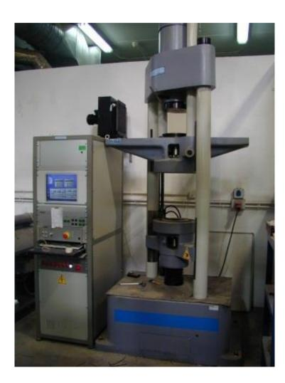
Universal testing machine, 600 kN load capacity:
