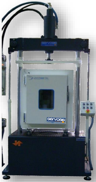
Climatic heat/cold chamber in universal testing machine model MUF 401
