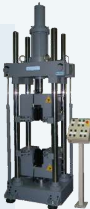
MUF 404/60 MACHINE WITH CH-4 ACTUATOR, MOUNTED ON UPPER BRIDGE.
