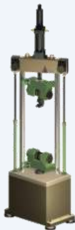
MUF 401 – C.S – B.A /10t Max force: 100 kN Bench on fsupporting rame. Upper actuator. Side action grip, model 4013
