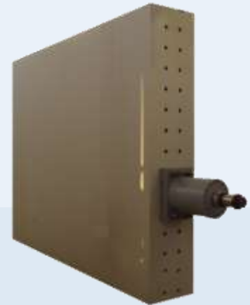
CH-4 1000 kN ACTUATOR HORIZONTAL MOUNTING ON A CONCRETE STRUCTURE, FOR WALL TESTS..
