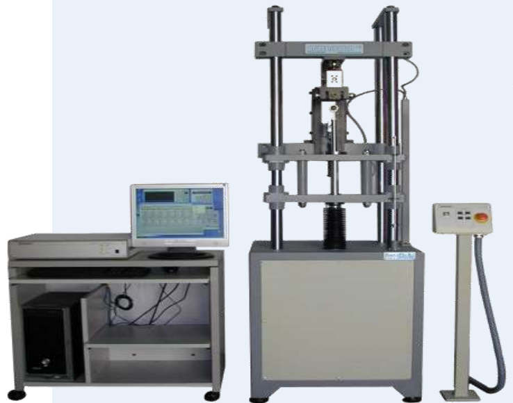
ME 402/5 kN with specific fixtures for shock absorber tubes tests.
