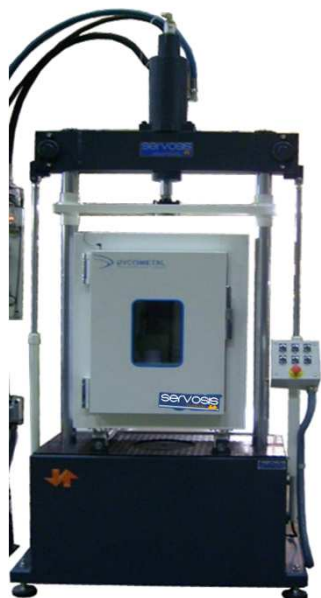
Climatic heat/cold chamber in universal testing machine model MUF 401
