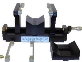
EN-12697-24. ANNEX E FATIGUE STRENGTH INDIRECT TENSILE STRENGTH OF CYLINDRICAL SPECIMEN. Fig E.1
