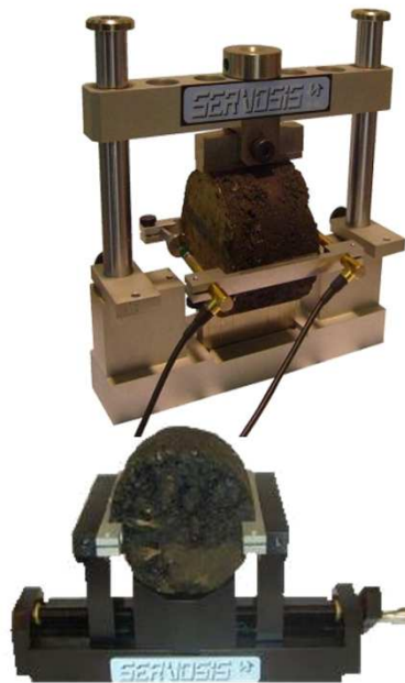
EN-12697-24. ANNEX E FATIGUE STRENGTH INDIRECT TENSILE STRENGTH OF CYLINDRICAL SPECIMEN. Fig E.1
